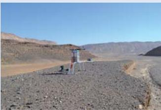
One approach for analysing the terrace surfaces is to describe single squaremeters documented with hyperspectral pictures using a RIKOLA hyperspectral Camera. This characterise the structure and colour of the desert pavement. Furthermore, the detailed recording of the hyperspectral signature serves as a ground check for analysing the satellite images (see figure 2).
