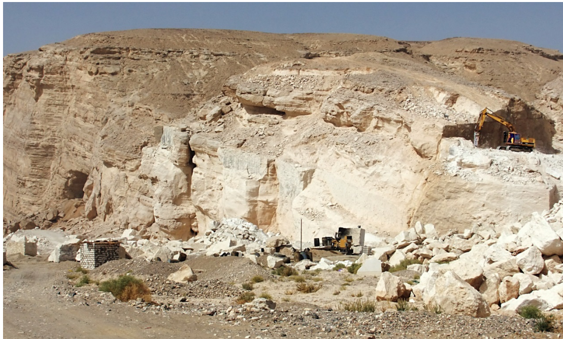
Figure 6. Actual status of the limestone quarrying in Wadi Sodmein, the cave entrance is clearly visible on the left hand side only a few meters away from the mining activities. Limestone is fractured directly on the spot.
