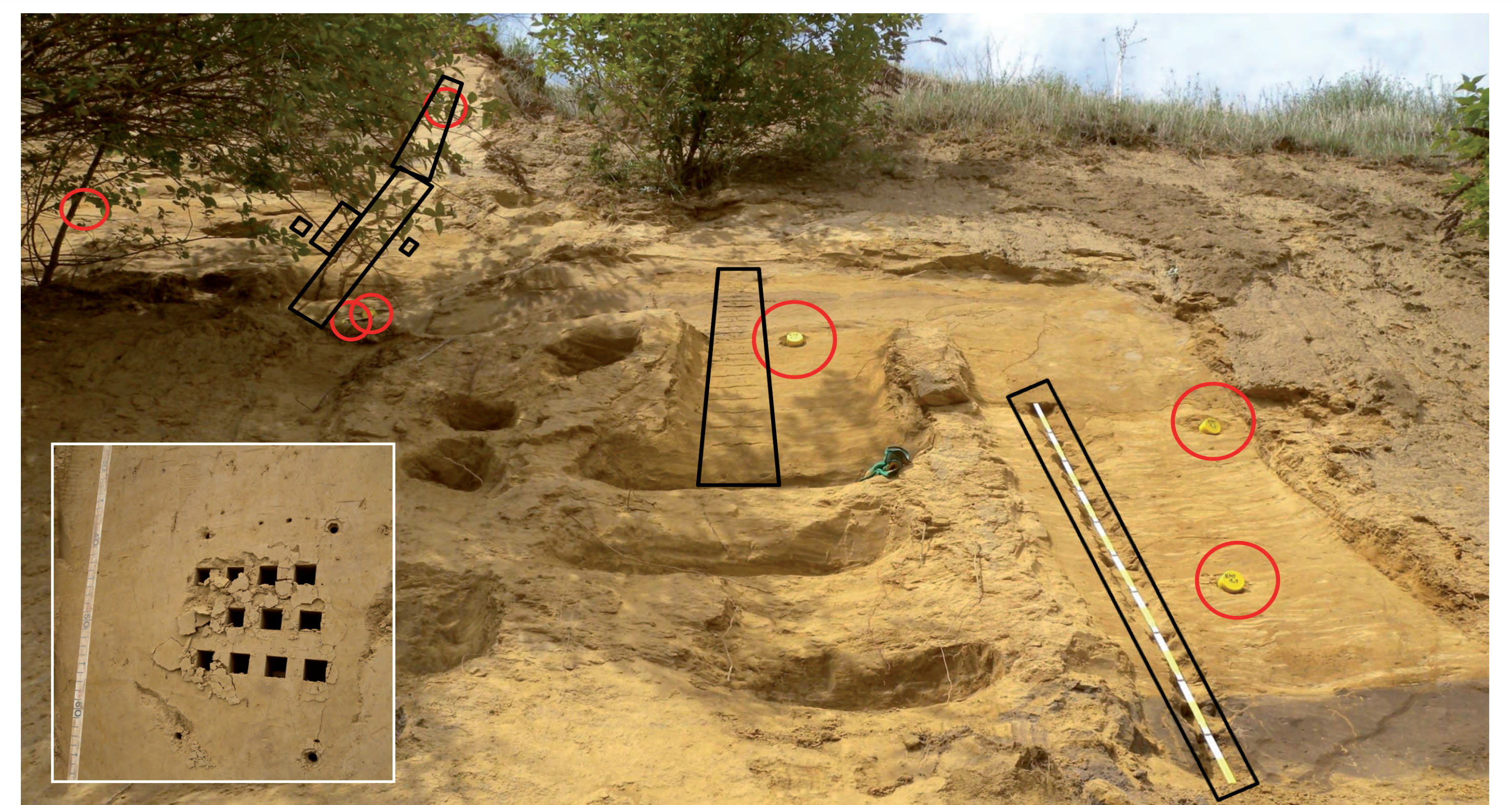
Fig.3 Quarry in Romont (Belgium): sampling for luminescence (red) and high resolution sampling for sedimentology and geochemistry (black); oriented sampling for AMS (small picture on the left)
