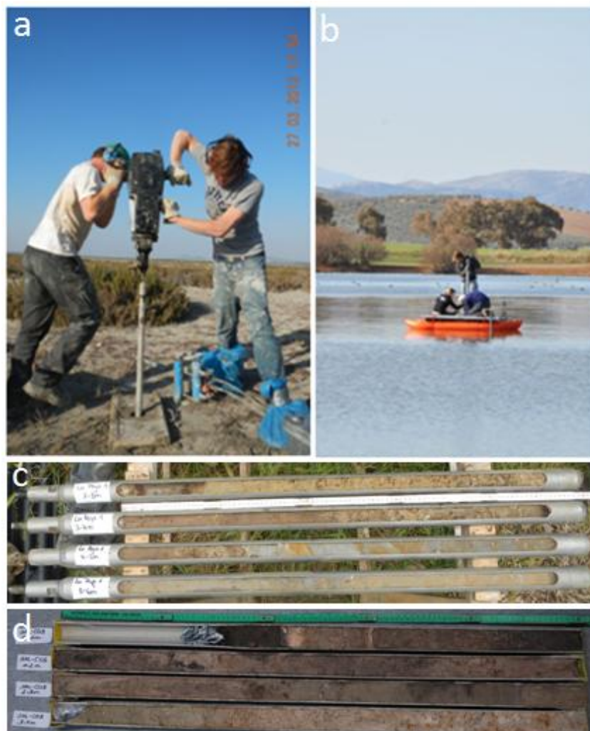
Fig. 17 Pictures of coring with a vibracorer (a), of the floating platform (b), the open drill probes (c) & halves of liner tubes (d)
