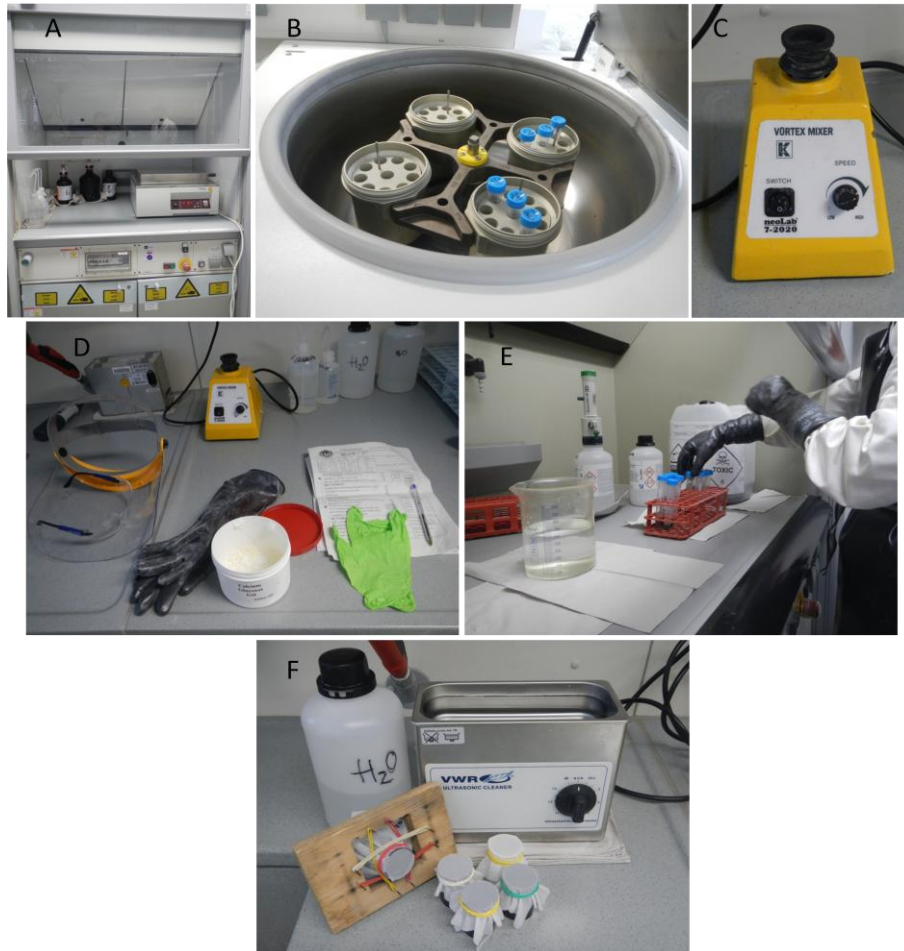
Fig. 23 (A) Picture of waterbath (middle right side of the picture), (B) centrifugal, (C) Vortex Mixer, (D) safety equipment for HF-treatment, (E) HF-treatment & (F) ultrasonic bath with preparation equipment
